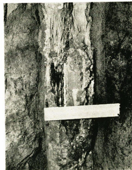
Above—Fig. 3: Diaphragm wall for underground car park in Berne with 111 temporary alluvium anchors. Below—Fig. 4: Grout cylinder formed in sand.
