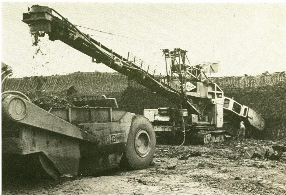
Fig. 4. O & K bucket wheel excavator digging London Clay and loading into a Cat 631B
