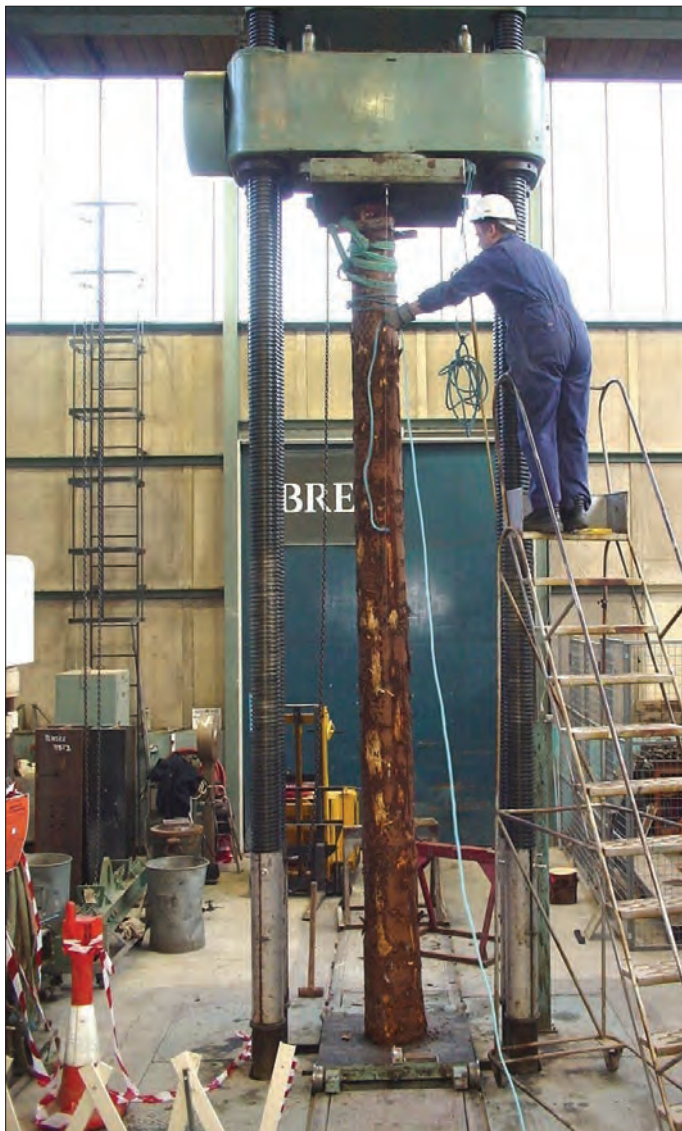
Figure 4: Axial load test on 4.6m log
